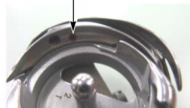
Lubrication hole (red mark)
